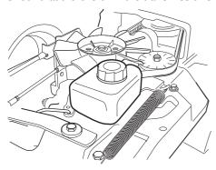
**Rider 318** Fill if necessary with engine oil SAE 10W/40 (class SF–CC).
